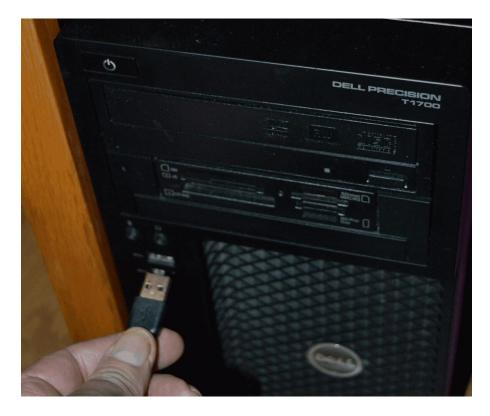
Then plug the large end of the USB cable into a spare port in your computer.
