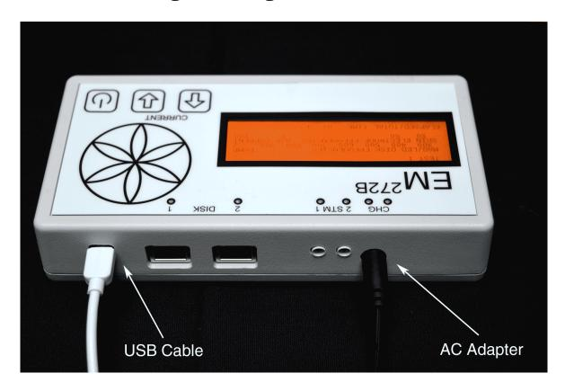
To program the **EM272B**<sup>TM</sup>, first connect the AC adapter to the device, plug it into a wall outlet, then turn the device ON.
