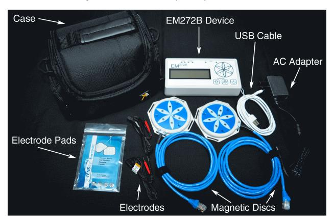
The **EM272B**<sup>TM</sup> comes in a kit with an **EM272B**<sup>TM</sup> device, a USB cable, an AC Adapter, two Magnetic Discs, two sets of Skin Electrodes, some Electrode Pads and a carrying case.
