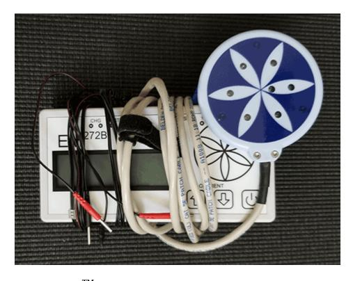
When storing the **EM272B**<sup>TM</sup>, you should never leave the Electrode cords and Magnetic Disc cords plugged into the device and then wrap them around the device as in the photo above. This puts a strain on the ends of the cords that plug into the device. Also, it puts strain on the 1/8" Electrode jacks and RJ45 Magnetic Disc jacks. This can cause damage to your unit.
